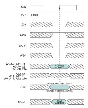
Figure 21: WRITE Burst
