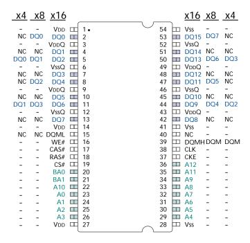
Notes: 1. The # symbol indicates signal is active LOW. A dash (-) indicates x8 and x4 pin function is same as x16 pin function.
