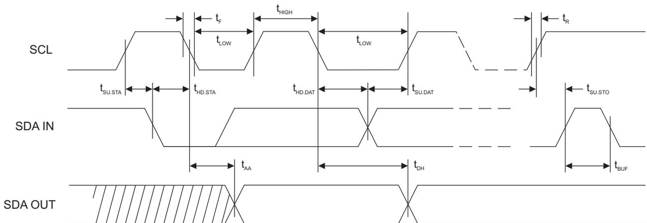
**Figure 6-3. Write Cycle Timing**
