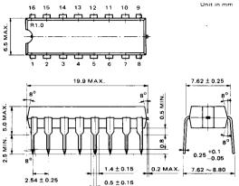
Note: Each lead pitch is 2.54mm. All leads are located within 0.25mm of their longitudinal position with respect to No. 1 and No. 16 leads.
