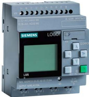
\*\*\*spare part\*\*\* SIPLUS LOGO! 12/24RCE based on 6ED1052-1MD08-0BA0 with conformal coating, -25...+60 °C, start up -20 °C, logic module, display power supply / I/O: 12/24 V DC/relay, 8 DI (4 AI)/4 DQ, memory 400 blocks, modularly expandable, Ethernet, integrated web server, data log, user-defined web pages, standard microSD card for LOGO! Soft Comfort V8 or higher, older projects executable
