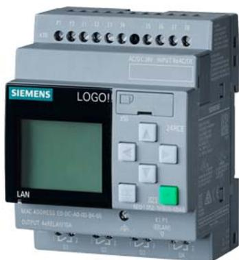
\*\*\*spare part\*\*\* SIPLUS LOGO! 24RCE based on 6ED1052-1HB08-0BA0 with conformal coating, -25...+60 °C, start up -20 °C, logic module, display power supply / I/O: 24 V AC/24 V DC/relay, 8 DI/4 DQ, memory 400 blocks, modularly expandable, Ethernet, integrated web server, data log, user-defined web pages, standard microSD card for LOGO! Soft Comfort V8 or higher, older projects executable
