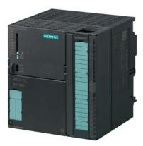
SIMATIC S7-300, CPU 317T-3 PN/DP, Central processing unit for PLC and technology tasks, 1024 KB work memory, 1st interface MPI/DP 12 Mbit/s, 2nd interface DP (drive), 3rd interface Ethernet PROFINET with 2-port switch, Integr. I/O for technology, Front connector (1x 40-pole) and Micro Memory Card min. 8 MB required
