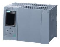
SIMATIC S7-1500H, CPU 1517H-3 PN, central processing unit with 2 MB work memory for program and 8 MB for data, 1st interface: PROFINET RT with 2-port switch, 2nd interface: PROFINET, 3rd/4th interface: H-SYNC, SIMATIC Memory Card required
