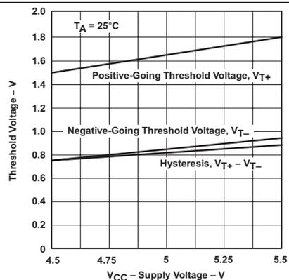
**Figure 12. Threshold Voltages and Hysteresis vs Supply Voltage**
