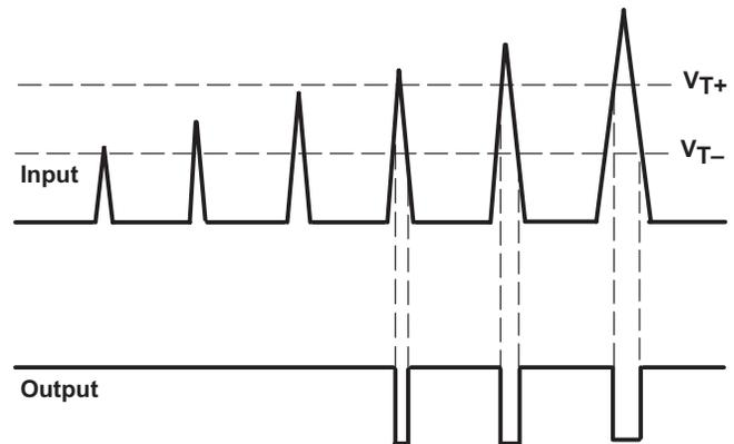
Figure 33. Threshold Detector
