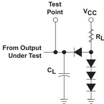
Figure 14. Load Circuit For 2-State Totem-Pole Outputs
