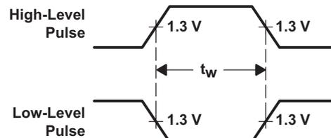
Figure 24. Voltage Waveforms Pulse Durations
