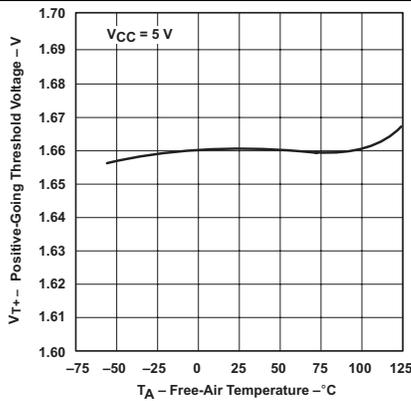
**Figure 8. Positive-Going Threshold Voltage vs Free-Air Temperature**
