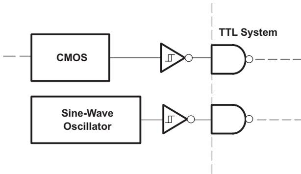
Figure 30. TTL System Interface For Slow Input Waveforms
