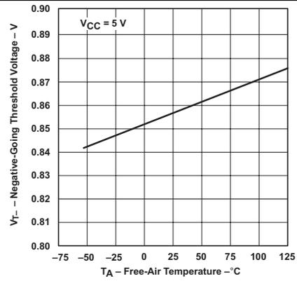
**Figure 9. Negative-Going Threshold Voltage vs Free-Air Temperature**
