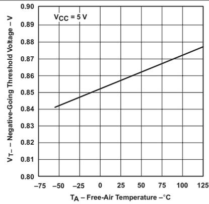
Figure 2. Negative-Going Threshold Voltage vs Free-Air Temperature
