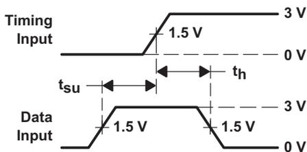
Figure 18. Voltage Waveforms Setup and Hold Times
