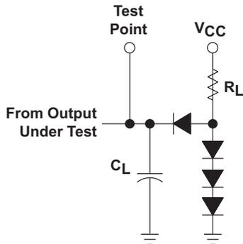
Figure 21. Load Circuit For 2-State Totem-Pole Outputs
