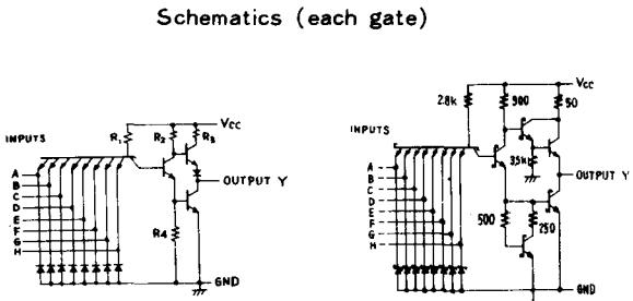
Input clamp diodes not on SN54L / SN74L circuits.
