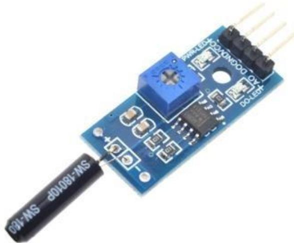
SW-18010P 3V to 5V Open Type Vibration Sensor Switch Module Alarm Trigger Geekcreit for Arduino - products that work with official Arduino boards
