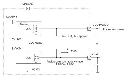
**Internal Power Supply Block Diagram**
