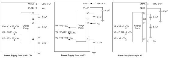
LCD Power Source from External Pin for C1 Type
