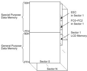
Note: 1. For HT67F5650, N=4 and the LCD Memory is from 80H~A7H; 2. For HT67F5660, N=8 and the LCD Memory is from 80H~AFH.
