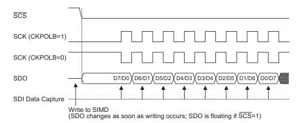
Note: For SPI slave mode, if SIMEN=1 and CSEN=0, SPI is always enabled and ignores the  $\overline{SCS}$  level.
