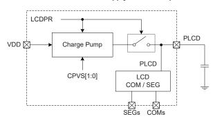
**LCD Driver Charge Pump Circuit**
