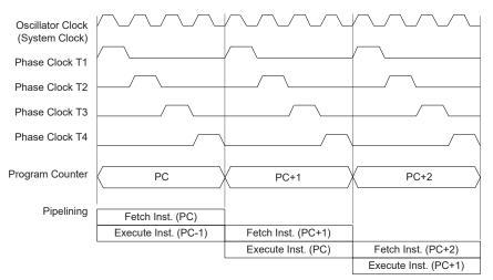
**System Clocking and Pipelining**
