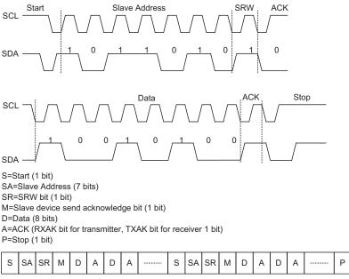
I<sup>2</sup>C Communication Timing Diagram
