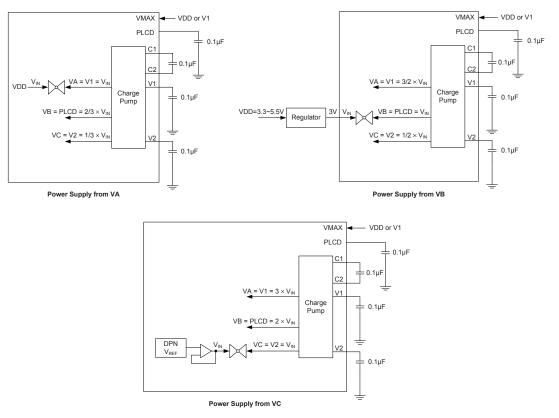
LCD Power Source from Internal Power for C2 Type
