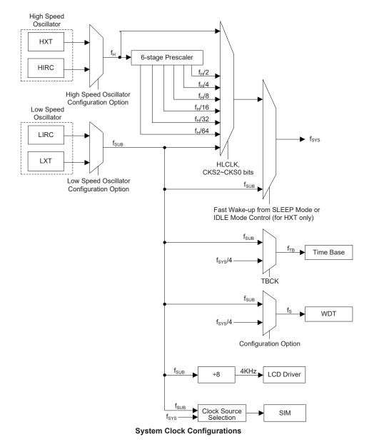
Note: When the system clock source  $f_{SYS}$  is switched to  $f_{SUB}$  from  $f_H$ , the high speed oscillation will stop to conserve the power. Thus there is no  $f_{H^{\sim}}f_H/64$  for peripheral circuit to use.
