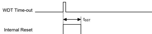
Note: The  $t_{SST}$  is 15~16 clock cycles if the system clock source is provided by ERC or HIRC.
