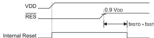
Note:  $t_{\text{RSTD}}$  is power-on delay, typical time=100ms
