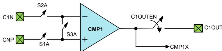
The following diagram and table illustrate the comparators switch control setting and the corresponding connections. Note that some switch control selections will force some switches to be controlled by hardware automatically.
