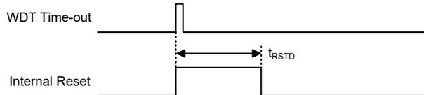
Note:  $t_{RSTD}$  is power-on delay, typical time=100ms
