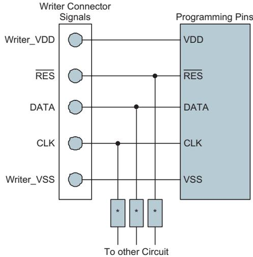
Note: \* may be resistor or capacitor. The resistance of \* must be greater than 1kΩ or the capacitance of \* must be less than 1nF.
