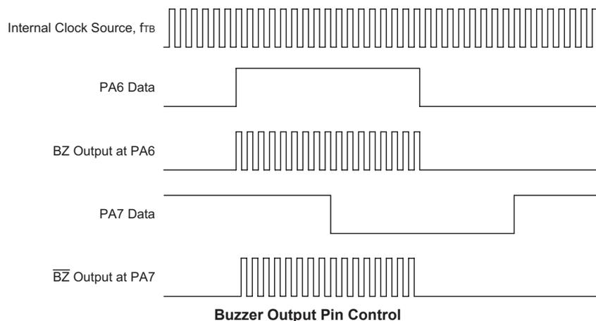
Note: The above drawing shows the situation where both pins PA6 and PA7 are selected by BPCTL option to be BZ and  $\overline{\text{BZ}}$  buzzer pin outputs. The Port Control Register of both pins must have already been setup as output. The data setup on pin PA7 has no effect on the buzzer outputs.
