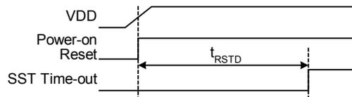
Note:  $t_{RSTD}$  is power-on delay, typical time=50ms
