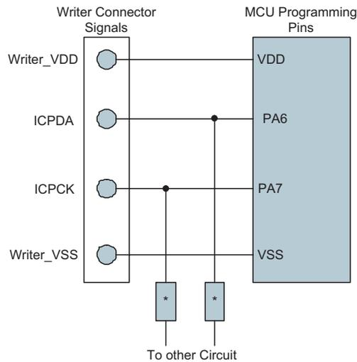
Note: \* may be resistor or capacitor. The resistance of \* must be greater than 1k or the capacitance of \* must be less than 1nF.
