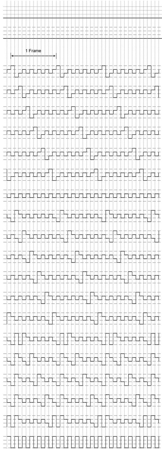
**LCD Driver Output – Type A, 1/6 Duty, 1/3 Bias**
