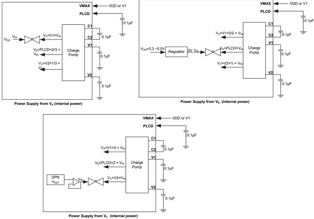
Note: The pin VMAX must connect to the maximum voltage to prevent from the pad leakage.
