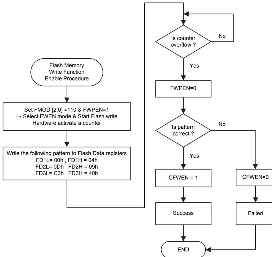
**Flash ROM Write Function Enable Procedure**
