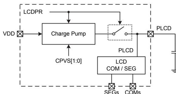
Note: when LCDPR=1, the external 4.7 $\mu$ F capacitor is required, when LCDPR=0, the capacitor can be removed.
