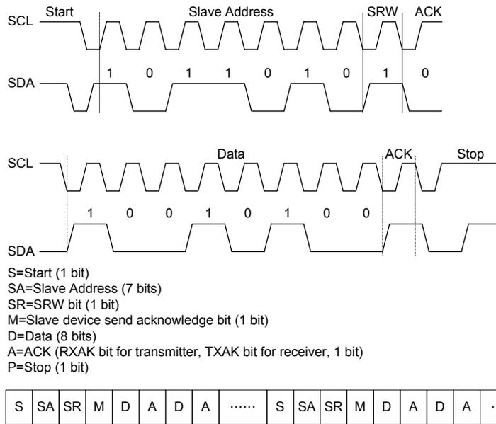
**I<sup>2</sup>C Communication Timing Diagram**
