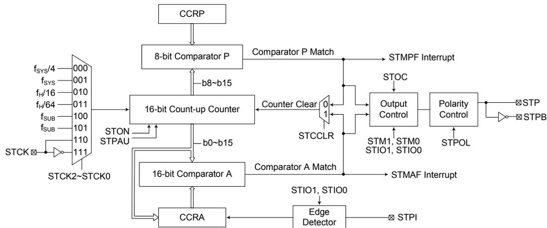
Note: The STM external pins are pin-shared with other functions and can input or output on different pins, so before using the STM function, the pin-shared function registers must be set properly.
