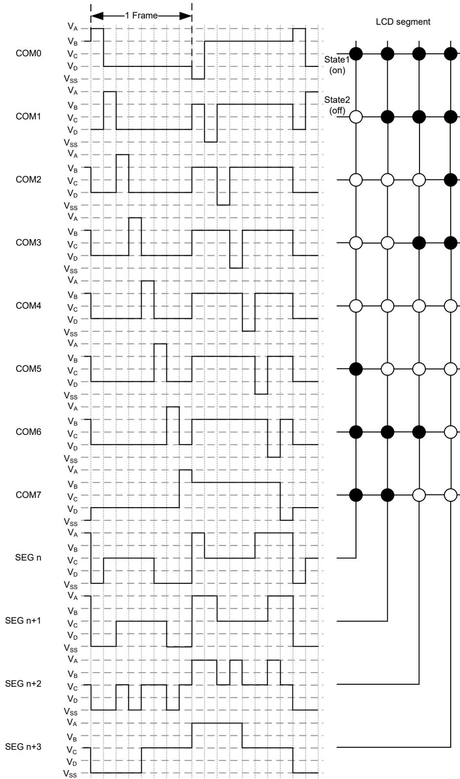
LCD Driver Output – Type B, 1/8 Duty, 1/4 Bias
