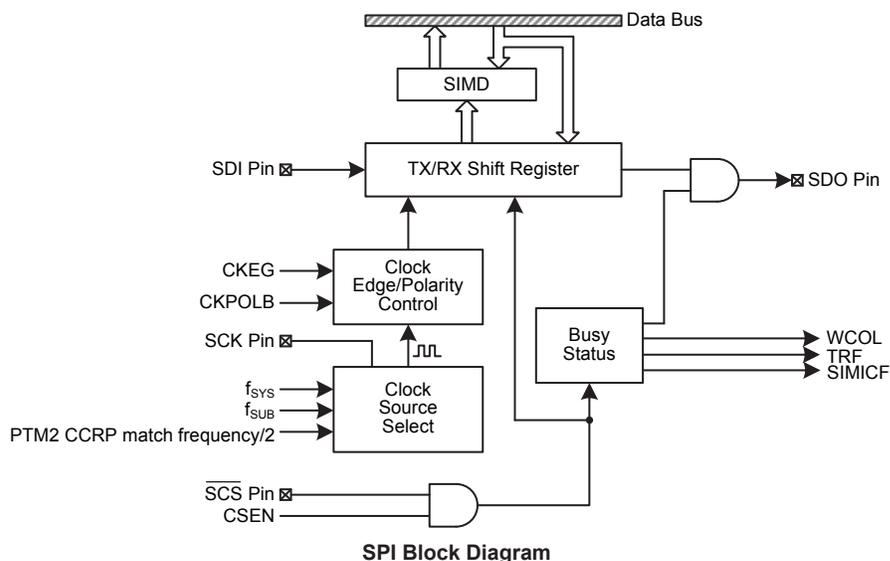
The SPI function in the device offers the following features:
