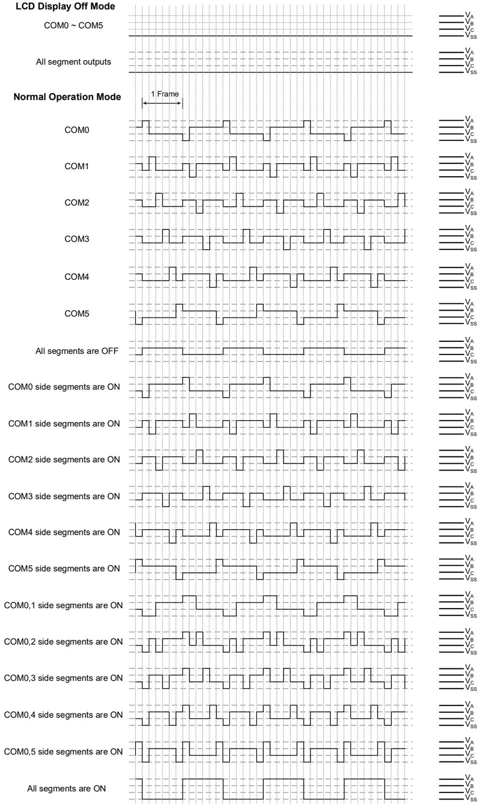
**LCD Driver Output – Type B, 1/6 Duty, 1/3 Bias**
