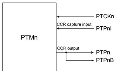
PTM Function Pin Control Block Diagram – n=0~2
