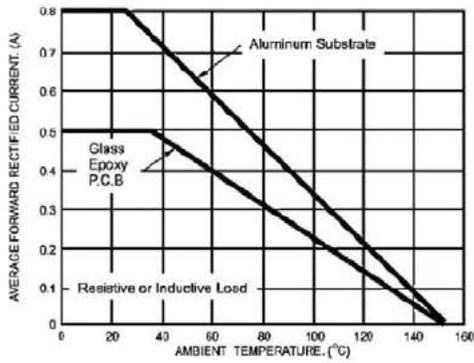
Figure 1. Derating Curve for Output Rectified Current
