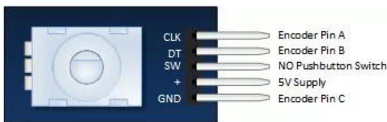
The module is designed so that a low is output when the switches are closed and a high when the switches are open.
