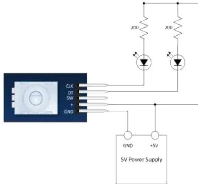
VERY SLOWLY rotate then encoder shaft both clockwise and counterclockwise. Notice which LEDs change state first with rotation.
