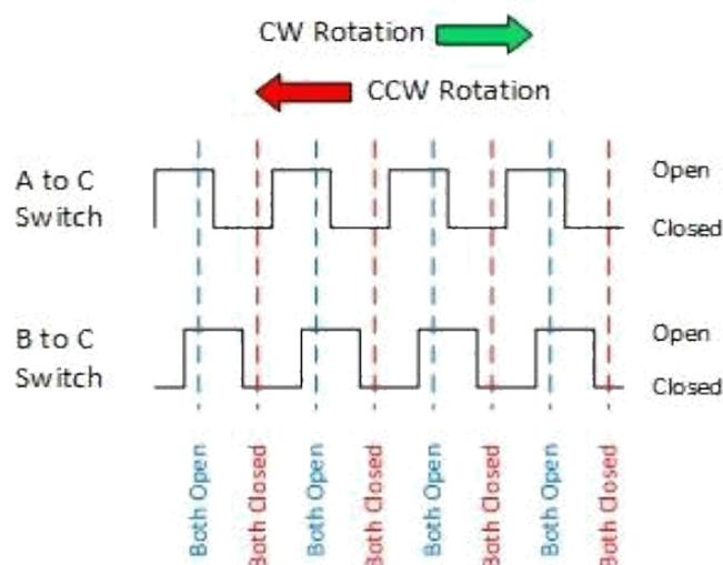
Essentially, determining which switch changed states first is how the direction of rotation is determined.
