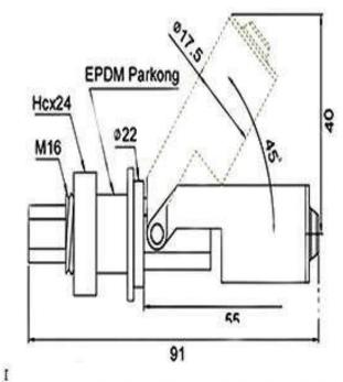
Float on the top, the level switch contacts normally closed
