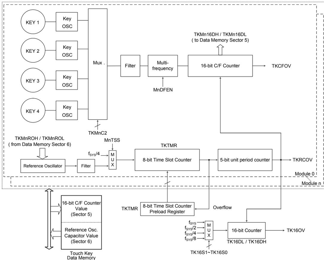
Note: The structure contained in the dash line is identical for each touch key module which contains four touch keys.
