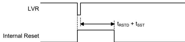
Note:  $t_{rSTD}$  is power-on delay with typical time=50ms
