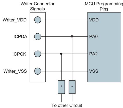
Note: \* may be resistor or capacitor. The resistance of \* must be greater than 1kΩ or the capacitance of \* must be less than 1nF.
