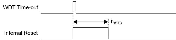
Note:  $t_{RSTD}$  is power-on delay with typical time=16.7ms
