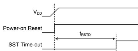
Note: t<sub>RSTD</sub> is power-on delay with typical time=50 ms
