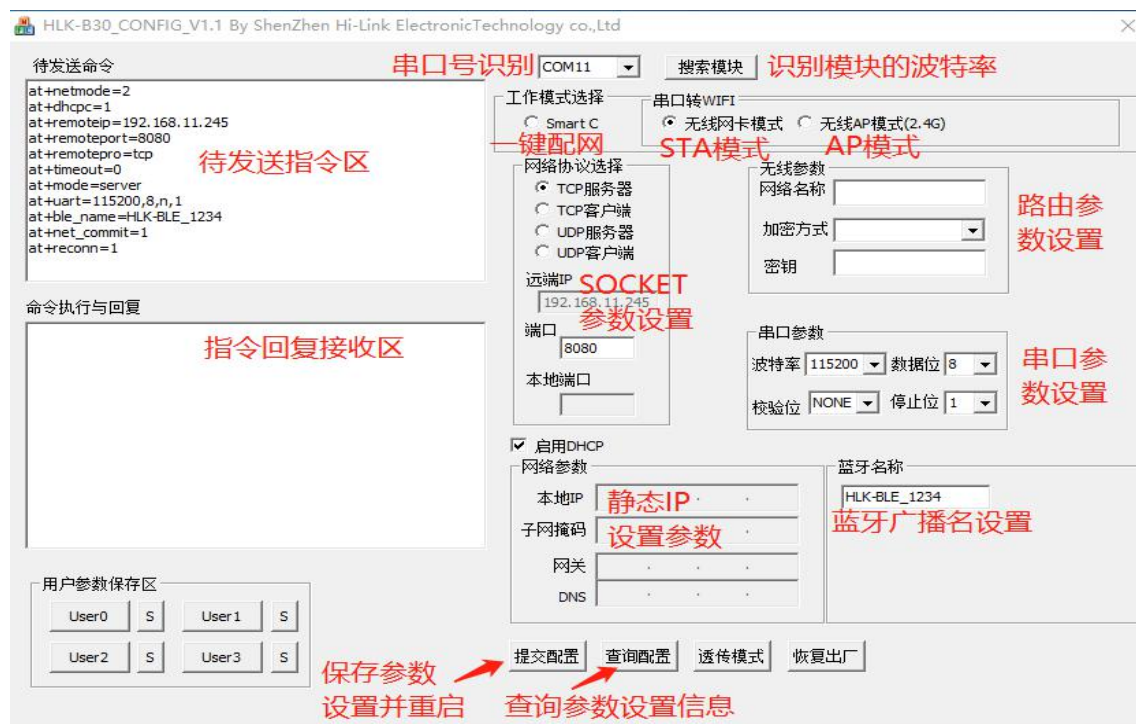
Pic 13 Serial port configuration interface
