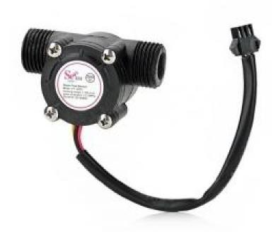
This sensor sits in line with your water line and contains a pinwheel sensor to measure how much liquid has moved through it. There's an integrated magnetic hall effect sensor that outputs an electrical pulse with every revolution. The hall effect sensor is sealed from the water pipe and allows the sensor to stay safe and dry.
