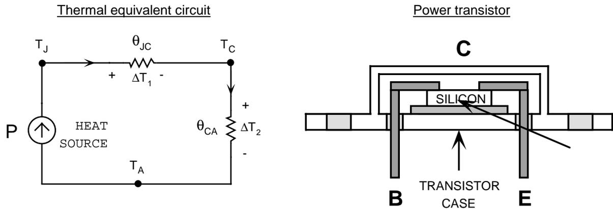
If the power dissipation of an electronic component is constant, it will heat up and reach thermal equilibrium, that is the silicon and case temperatures will reach constant levels. Under those conditions, we can use thermal Ohm's law to calculate the steady-state temperatures.
