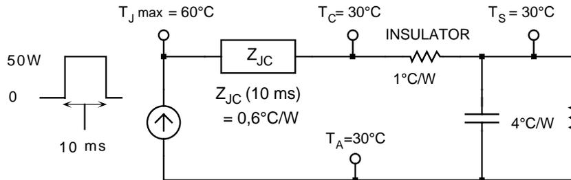
The thermal time constant from junction to case can be obtained from the 0% duty cycle curve: after one  $\tau_{JC}$ ,  $r(t) = (1 - e^{-t/\tau}) = 0,632$  and we read  $t = \tau_{JC} = 75$  ms.
