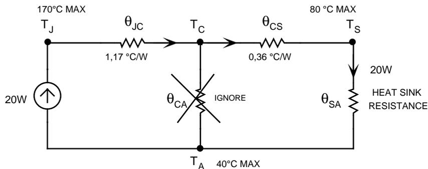
$$T_J = T_A + P \times \theta_{tot} < 140 \Rightarrow \theta_{tot} < \frac{T_{J,max} - T_A}{P} = \frac{140 - 40}{20} = 5 \text{ }^\circ\text{C/W}$$
