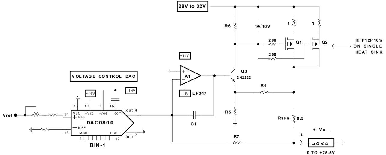
The worst case power dissipation for the MOSFETs is when  $V_{DS}$  is maximum which occurs when  $V_o$  is 0V and  $I_L = 2.55A$  max.
