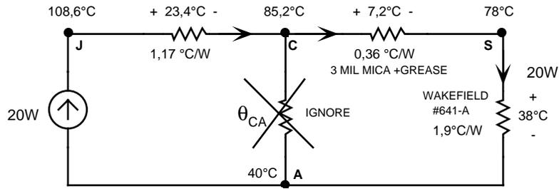
C) Assuming again that a Wakefield #641-A heat sink is used, determine  $T_J$ ,  $T_C$  and  $T_S$  for an ambient temperature of  $40^\circ\text{C}$  when 20W is dissipated. Assume that forced-air convection (a fan) is used with an air velocity of 150 FPM (feet per minute).
