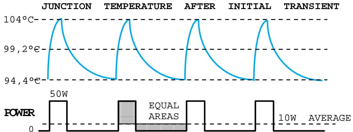
The above calculations show that  $T_J$  max is well below the maximum 200°C specified. After ensuring operation within the FBSOA the device is deemed to operate safely.
