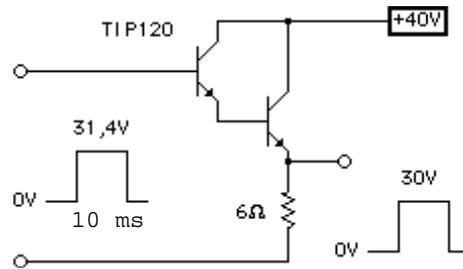
We can read  $r(t) = 0,31$  at  $t = 10$  ms on the transient thermal impedance shown at the bottom of the previous page. (for TIP120)
