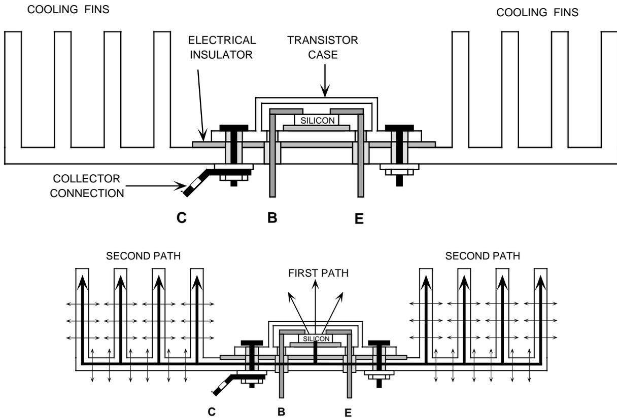
FIRST PATH: JUNCTION TO CASE TO AMBIENT AIR, HIGH RESISTANCE PATH
