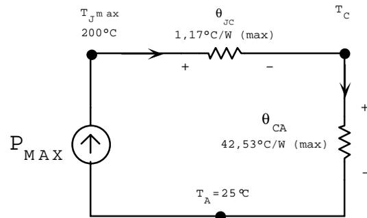
This maximum power can only be achieved if we mount the transistor on an infinite heat sink whose thermal resistance is zero. This is physically impossible and costly. In practice heat sink thermal resistances can be as low as 0,25 °C/W but the heat sinks become physically quite large.
