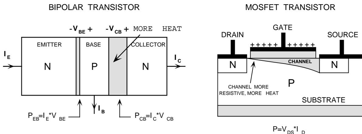
In a bipolar transistor most of the heat is generated at the CB junction where the voltage drop is higher. Therefore the collector usually makes a physical contact with the transistor case for better heat transfer to the ambient air surrounding the case - the metal case is a good heat conductor.
