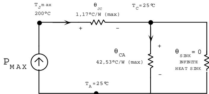
B) What is the maximum power that can be dissipated without a heat sink at ambient temperatures of +25°C and +50°C?
