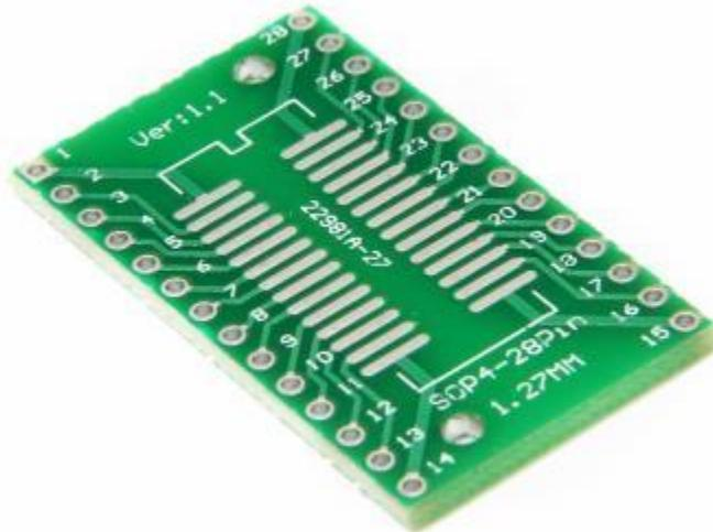
TSSOP28 SSOP28 SOP28 SMD to DIP28 IC Adapter Converter Socket Board Module Adapters Plate 0.65mm 1.27mm Integrate
