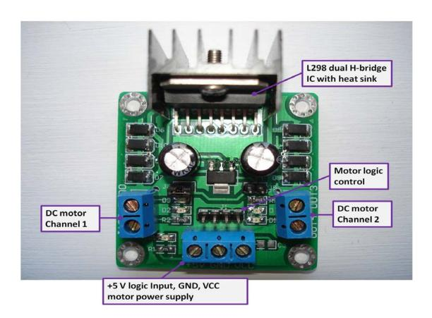
This article explains how the +5 V and Vcc of this motor controller work.
