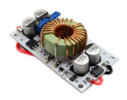
250W Boost Converter DC/DC 8.5-48V to 12-50V Output Step-up Module Mobile Power Supply Max 10A
