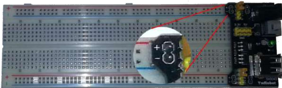
Make sure that you align the module correctly on the breadboard. The negative pin(-) on module lines up with the blue line(-) on breadboard and that the positive pin(+) lines up with the red line(+). Failure to do so could result in you accidentally reversing the power to your project.
