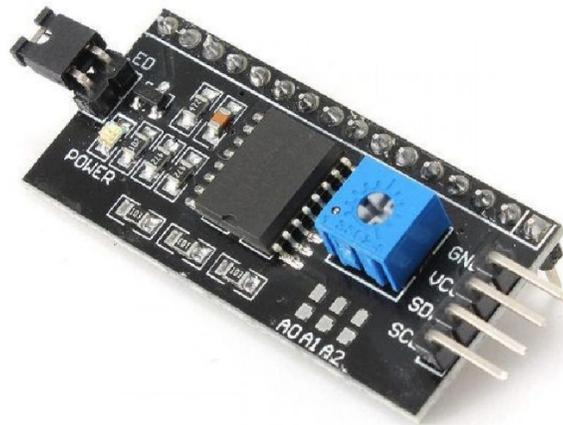
Interface Adapter Plate LCD1602 IIC/I2C is an LCD interface adapter for Arduino without the LCD screen. Since Arduino board I/O ports are limited using Interface Adapter Plate LCD1602 IIC/I2C will let you add extra devices to your Arduino board. The module supports I2C protocol and the LCD contrast can be adjusted using the potentiometer on the board.
