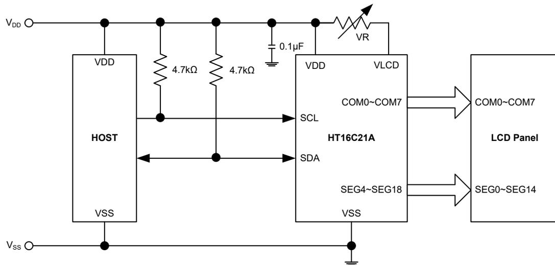
When the internal  $V_{LCD}$  voltage adjustment function is enabled and the Segment/VLCD shared pin is set as VLCD pin, the bias voltage is supplied by the internal adjusted voltage, derived from the  $V_{DD}$  voltage, determined by the DA3~DA0 bits and the VLCD pin is used as an output pin of which the voltage is detected by the external MCU host.
