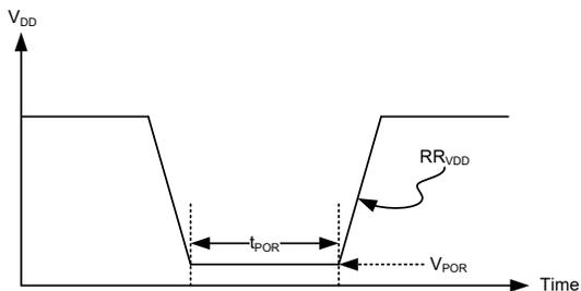
Note that if the power-on reset timing conditions are not satisfied during the power on/off sequence, the internal power-on reset circuit will not operate normally. Also if  $V_{DD}$  drops below the minimum voltage of operating voltage specification during operation, the power-on reset timing conditions must be also satisfied. This means that  $V_{DD}$  must fall to 0V and remain at 0V for a minimum time of 10ms before rising to the normal operating voltage.
