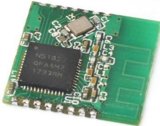
**Low power Bluetooth BLE4.0 main module TTL serial port transparent transmission Nordic igyro nRF51822**
