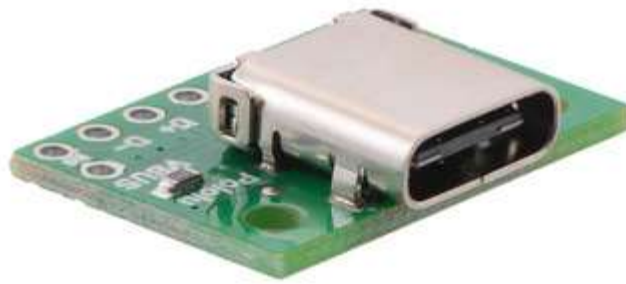
Close-up of Type-C connector on the USB 2.0 Type-C Connector Breakout Board.
