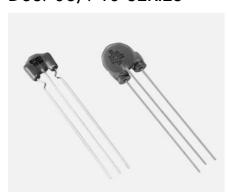
The DSS706 Varistor-Capacitor is a three-terminal filter which suppresses noise emission from electronic equipment while controlling incoming surges of static electricity. Its small size enables 2.5mm pitch mounting.
