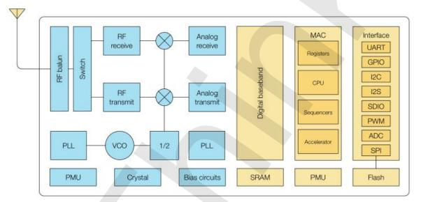
The ESP8266 is a complete and self-contained WiFi network solution that can operate independently or as a slave running on other host MCUs. The ESP8266 is capable of booting directly from an external flash memory when it is powered by an application and is the only application processor in the device. The built-in cache helps improve system performance and reduce memory requirements.
