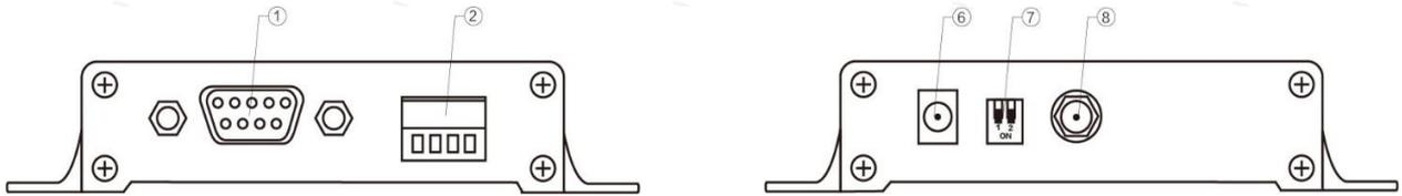
Users can choose ⑥ DC power interface, using the power adapter supply with the interface of the 5.5mm outer diameter, 2.5mm diameter;
