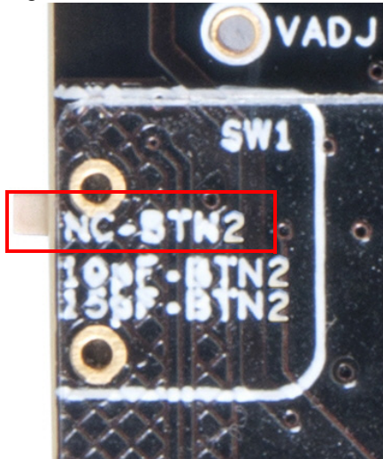
Figure 3-19. SW1 Slide Switch in NC-BTN2 Position
