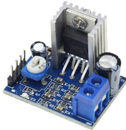
TDA2030 Audio Amplifier module is based on the TDA2030 audio amplifier chip, which is capable of 18 W output power with low harmonic distortion.
