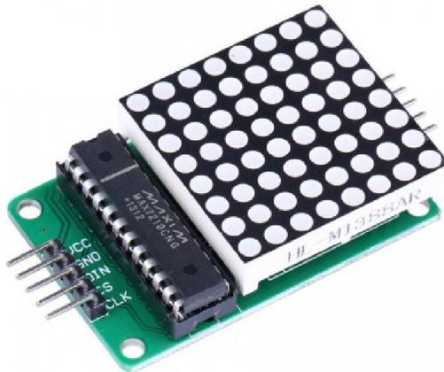
MAX7219 is a kind of integrated serial input/ output common cathode display driver, it connects microprocessor and 8-digit seven period of digital LED display, also can be connected to the bar graph display or 64 independent LED.
