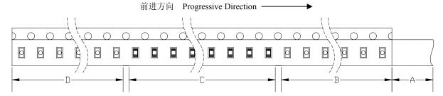
A: 盖带, 300 mm; B: 引导, 空带, 200mm; C: 编载产品 3000 只; D: 尾部, 空带, 200mm A: Top Cover Tape, 300mm; B: Leader, Empty, 200mm; C:3000 Lamps Loaded; D: Trailer, Empty, 200mm.
