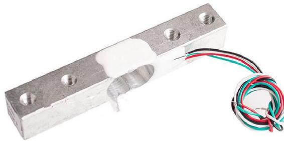
Electronic weighing machine uses load cell to measure the load or pressure produced by the load, here most load cells are follows the method of strain gauge, Which converts the pressure (force) into an electrical signal, these load cells have four strain gauges that are hooked up in a Wheatstone bridge formation.
