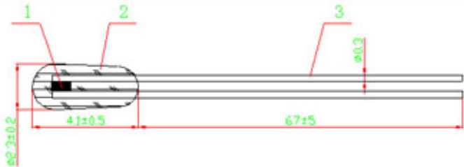
MF58J • 1---chip, 2---glass encapsulation, 3---lead wire
