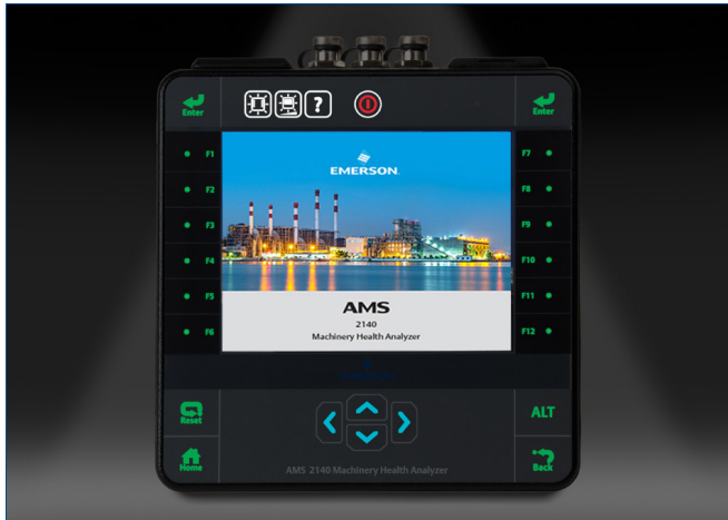
The backlit keypad and ambient lighting of the larger, brighter screens makes the AMS 2140 visible in any environment.
