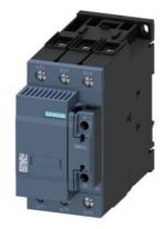
capacitor contactor, AC-6b 50 kVAr, / 400 V, 3-pole, 230 V AC, 50 Hz, auxiliary contacts: 1 NO + 1 NC, screw terminal, size: S2  $\,$
