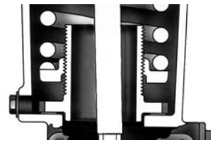
Figure 1. Sectional Views of Spring Seat Construction Details
